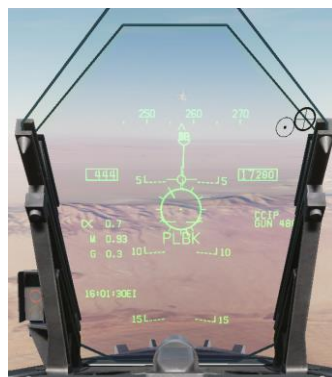
Figure 131. "PLBK" label displayed when Pullback is inhibited.
