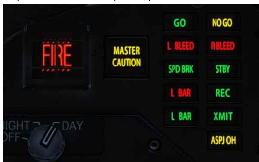
Figure 236. ASPJ annunciator panel
