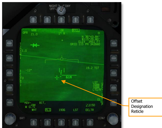
Figure 221. Offset Designation Reticle
