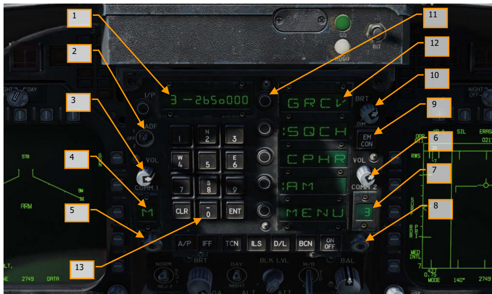
Figure 11. Up-Front Controller
