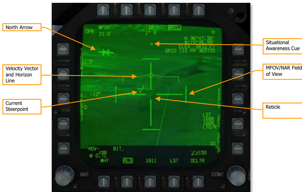
Figure 217. ATFLIR format in OPR mode (display elements).
