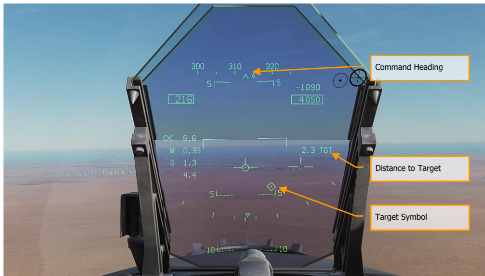
Figure 50. Waypoint as Target on HUD
