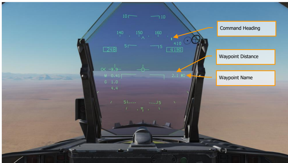
Figure 49. Waypoint Steering on HUD
