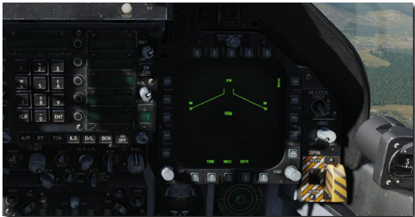
Figure 39. Stores Management System (SMS) Page
