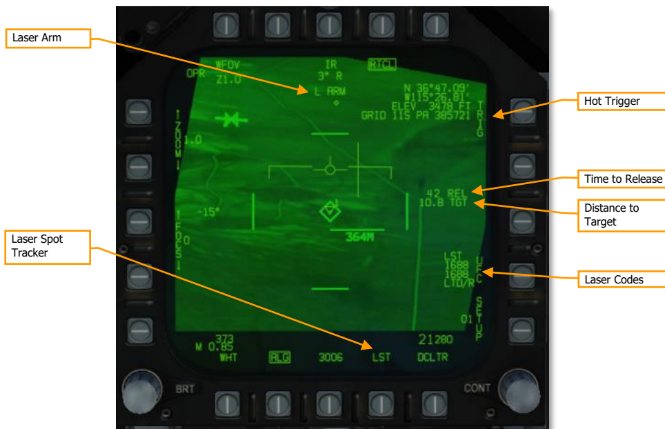
Figure 219. ATFLIR LTD/R and LST controls.
