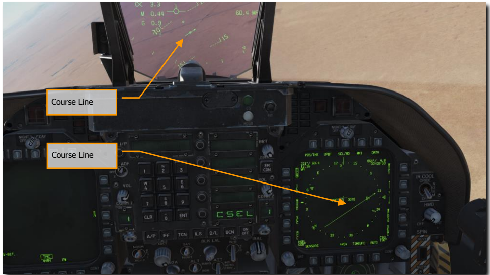
Figure 75. Course Setting on HSI and HUD
