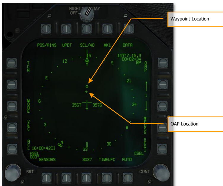
Figure 63. Offset Aimpoint on HSI
