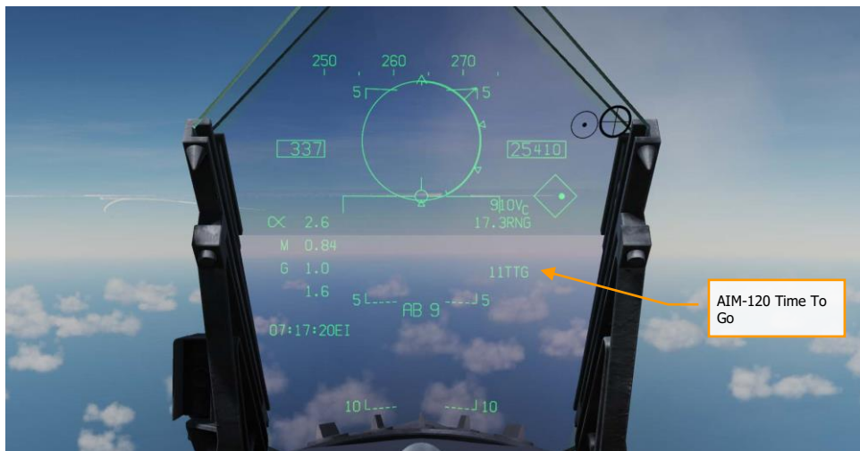
Figure 203. AIM-120 Radar Tracking, Post Launch HUD
