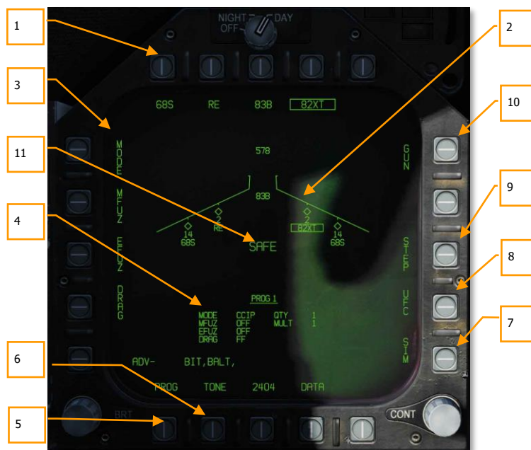
Figure 83. A/G Conventional Bombing SMS Page
