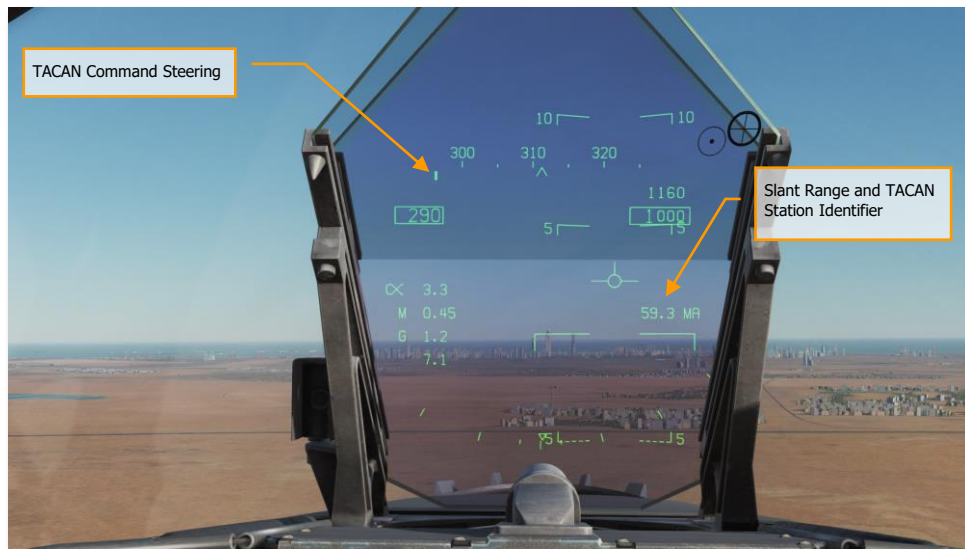
Figure 69. TACAN Steering on HUD
