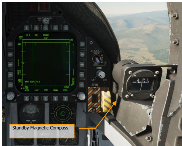
Figure 23. Standby Magnetic Compass
