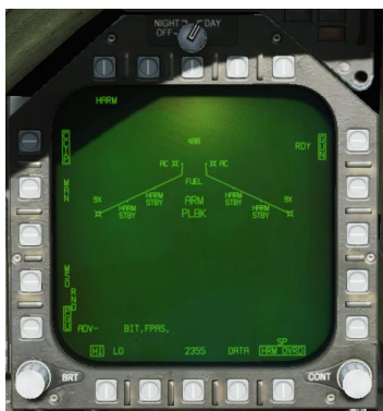
Figure 131. "PLBK" label displayed when Pullback is inhibited.
