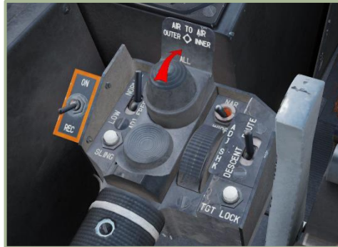
11-14: Hardpoint selector set to AIR TO AIR
