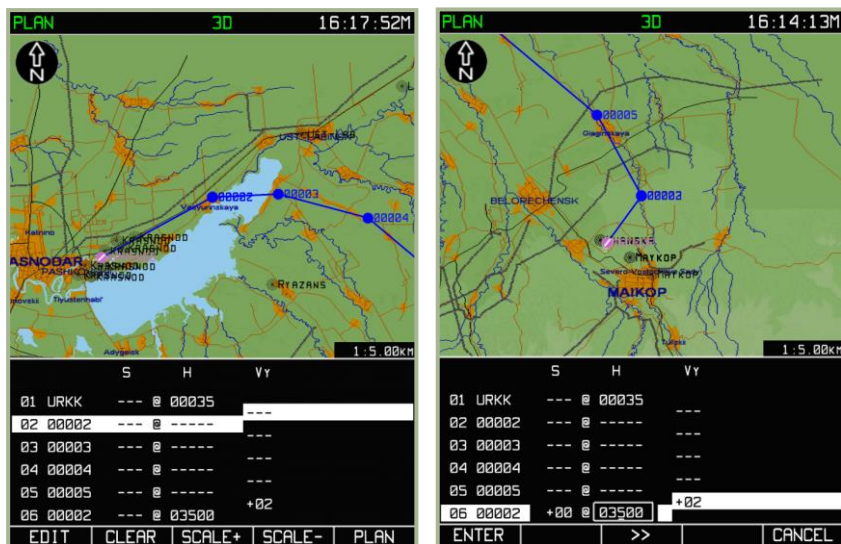
7-53: Clearing flight altitude values for the intermediate altitudes
