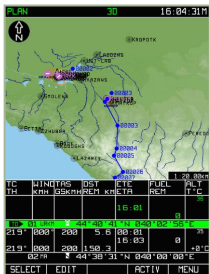
7-69: PLAN sub-mode after route is loaded
