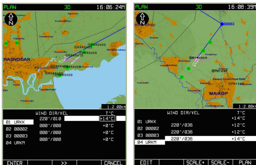
7-58: Example of entering ambient temperature value
