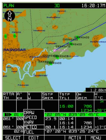
7-56: Selecting the METEO sub-mode from MENU/PLAN sub-mode
