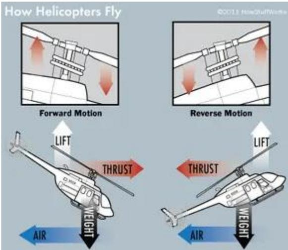
Flying a helicopter is more intricate than piloting an airplane due to the constant management of flight controls. Unlike airplanes, helicopters have the ability to move backwards, sideways, and hover in place.
