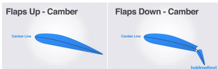
Flaps are used to reduce the speed of the aircraft while increasing lift.
