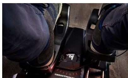
In some aircraft, the rudder pedal also functions as the left and right wheel brakes, similar to a car pedal that is pressed with the toes.
