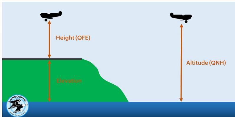
The **QFE** represents the current atmospheric pressure at the airfield, while the **QNH** is the atmospheric pressure adjusted to sea level. It is important to note that these values are influenced by various factors such as temperature and wind, making them specific to each location and variable.
