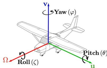
The joystick is responsible for controlling the **Pitch** and **Roll** of the aircraft, while the pilot's feet operate the rudder pedals to control the **Yaw** axis. For instance, when the pilot needs to move the aircraft to the right, he push with his right foot and simultaneously move his left foot back.
