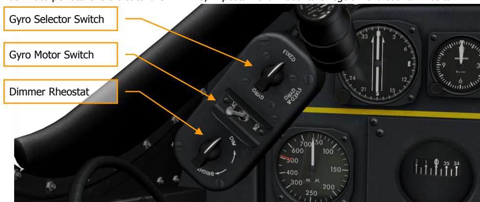
Figura 37: K-14A Pannello Mirino Selector-Dimmer
