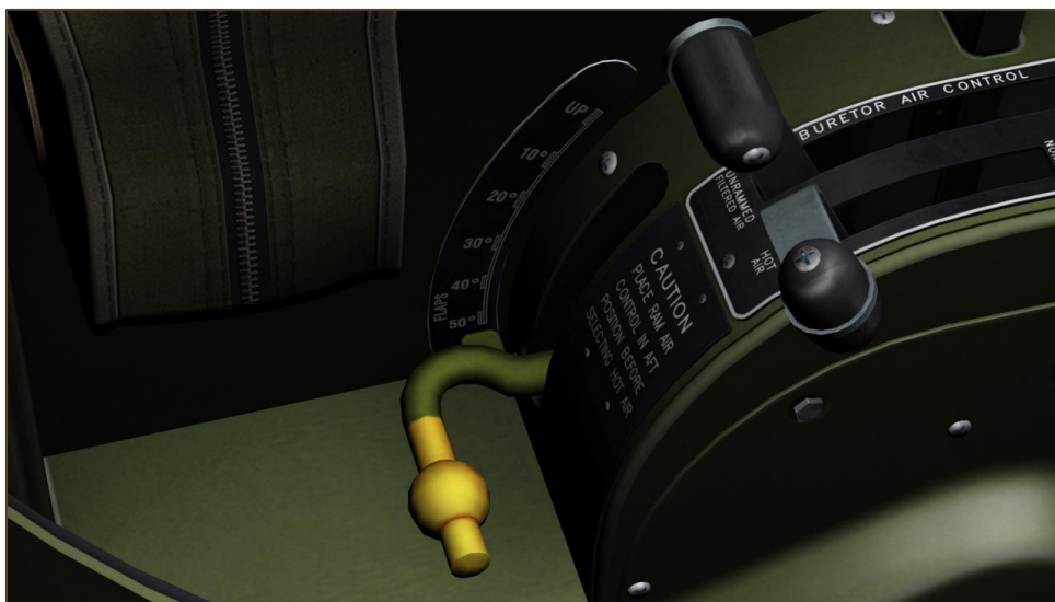
Figura 68: Controlli Flaps
