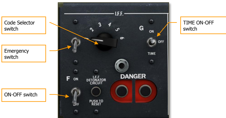
Figura 77: SCR-695-A IFF Radio
