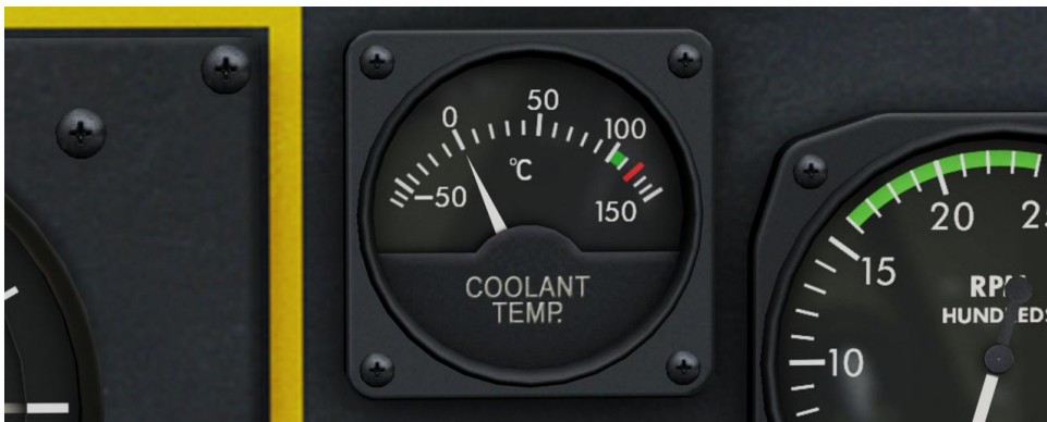
Figure 86: Massima temperatura refrigerante 121°C (250°F), limiti operativi 100...110°C (212...230°F)
