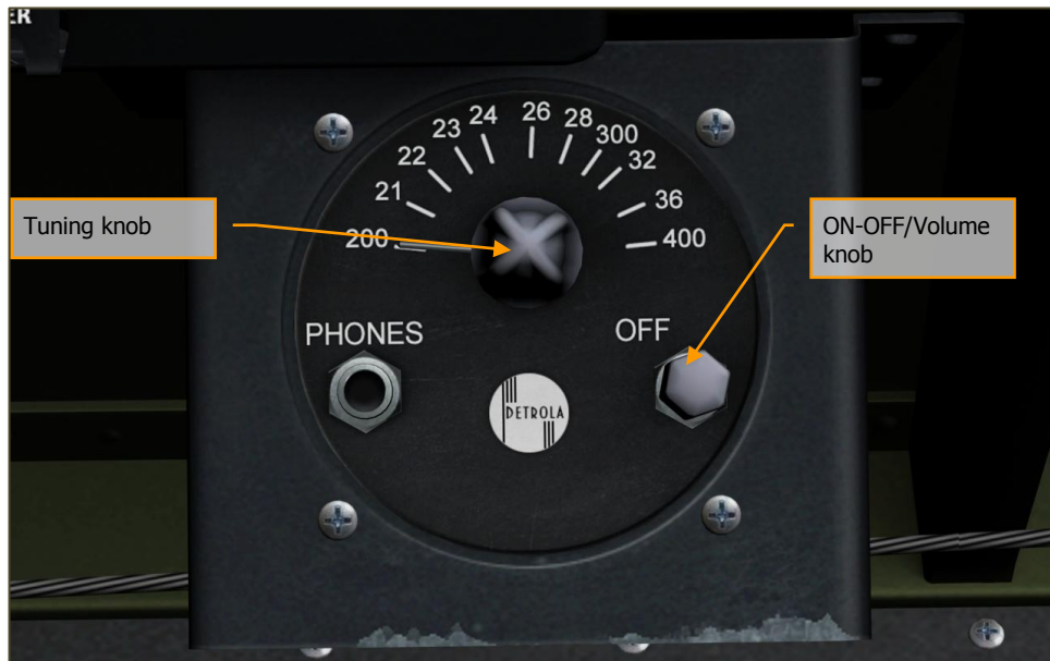
Figura 79: BC-1206 "Detrola" Radio Range Receiver
