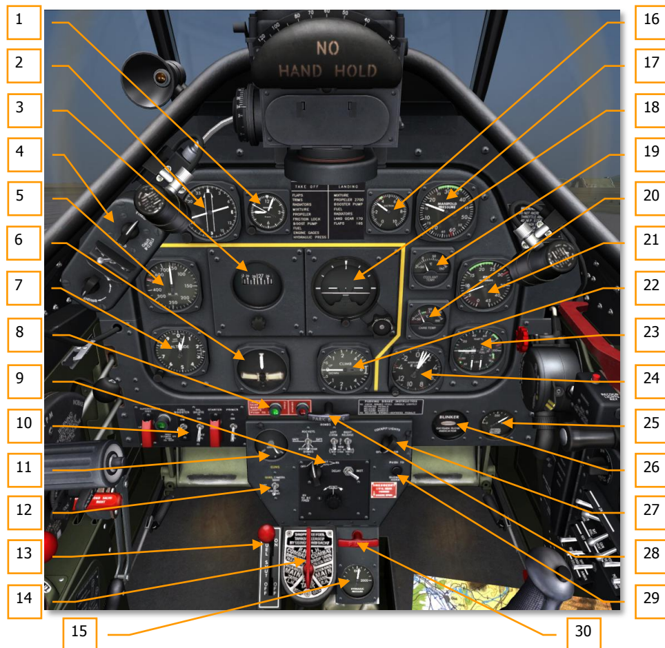
Figura 32: P-51D console frontale cockpit
