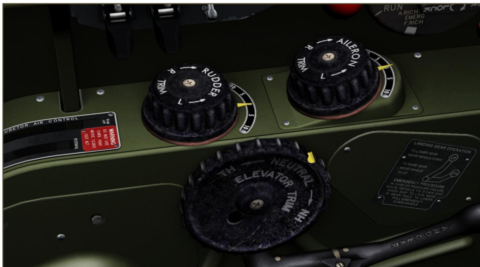
Figure 66: Trim Tab Controls
