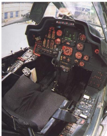
Aft cockpit of the AH-64A with analog gauges and switches (Left) and the aft cockpit of the AH-64D featuring the MANPRINT cockpit design and layout (Right) (US Army)
