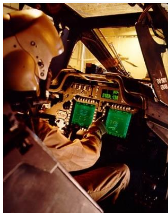
Aft cockpit of the AH-64A with analog gauges and switches (Left) and the aft cockpit of the AH-64D featuring the MANPRINT cockpit design and layout (Right) (US Army)
