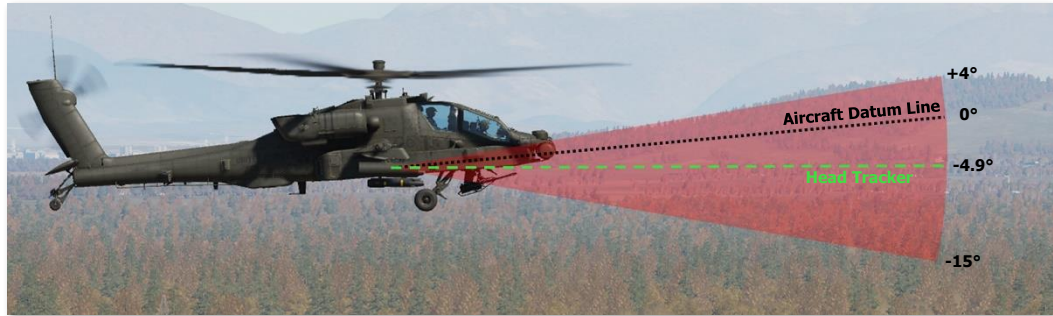
Pylon Articulation Limits
