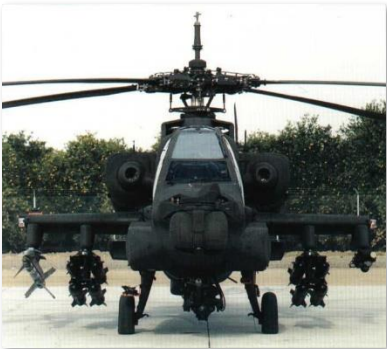
AH-64A mock-up with Sidewinder and ATAS missile systems (McDonnell Douglas)
