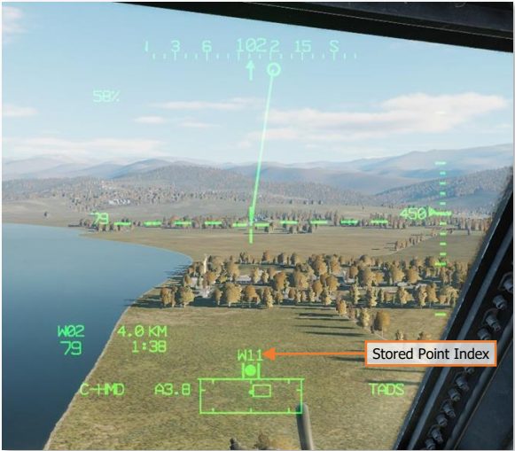
Storing a point using the HMD line-of-sight
