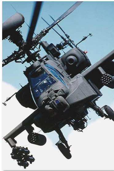
AH-64D equipped with the mast-mounted AN/APG-78 Fire Control Radar (US Army)
