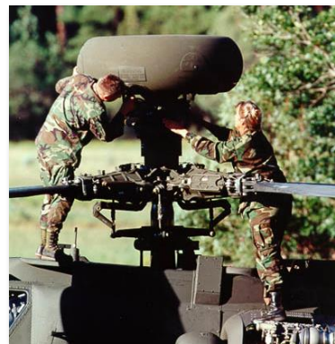
Maintenance personnel inspect an AH-64D's mast-mounted assembly (US Army)
